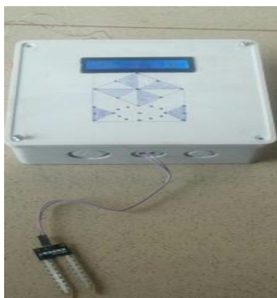
Figure 10: Developed wireless sensor node after packaging with battery.
